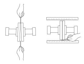
Figure 6. Aligning Non-Spider Type Couplings
